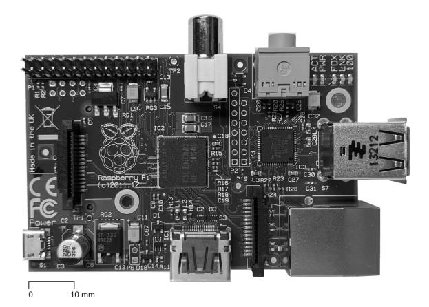
As for microcontrollers, single-board computers are difficult to maintain as components are soldered directly onto the circuit board and are not easily replaceable. The recoverability of code and other stored data is highly dependent on the device and nature of the storage medium. Data may be retrievable where it is contained on removable storage media (e.g., an SD card or USB stick), but storage integrated into the board may be very difficult to access.
